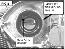
Refer to PIC 5. Align the black plastic Dual Velocity ring with the Hypercharger vent hole. Press it all the way into place. The ring will "snap" into place.
