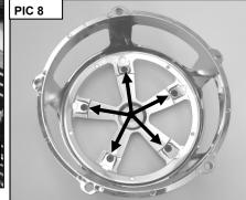
**STEP 16** As shown in PIC 10, Align the Mach 2 Ring Adapter with the front side of the Cover; secure using the five (5) small screws from the backside.
