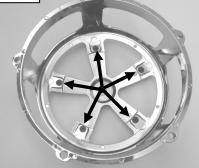
PIC 9 As shown in PIC 10, Align the Mach 2 Ring Adapter with the front side of the Cover; secure Install the screen inside the Mach 2 Cover; place the cover over the Filter Element.
