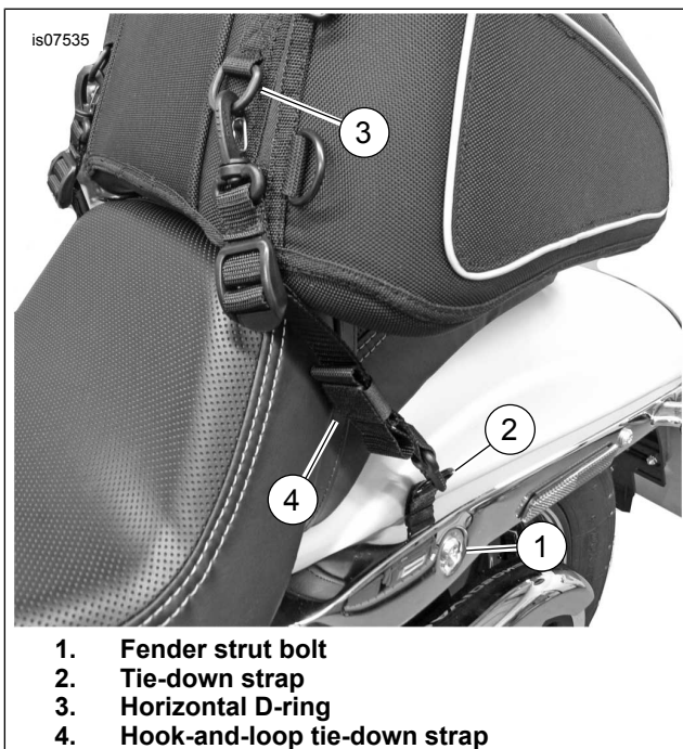
Figure 3. Front Strap Installation (Sportster, Dyna, Softail)
