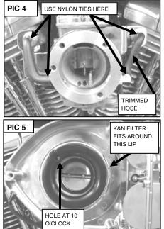
**STEP 11** Refer to **PIC 5.** Align the black plastic Dual Velocity ring with the Hypercharger vent hole. Press it all the way into place. The ring will "snap" into place.
