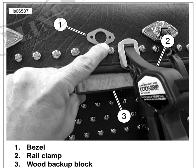
Figure 2. Using the bezel as a template
