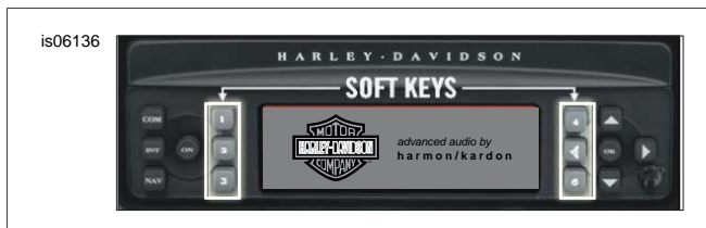
Figure 2. Advanced Audio Receiver "Soft" Keys
