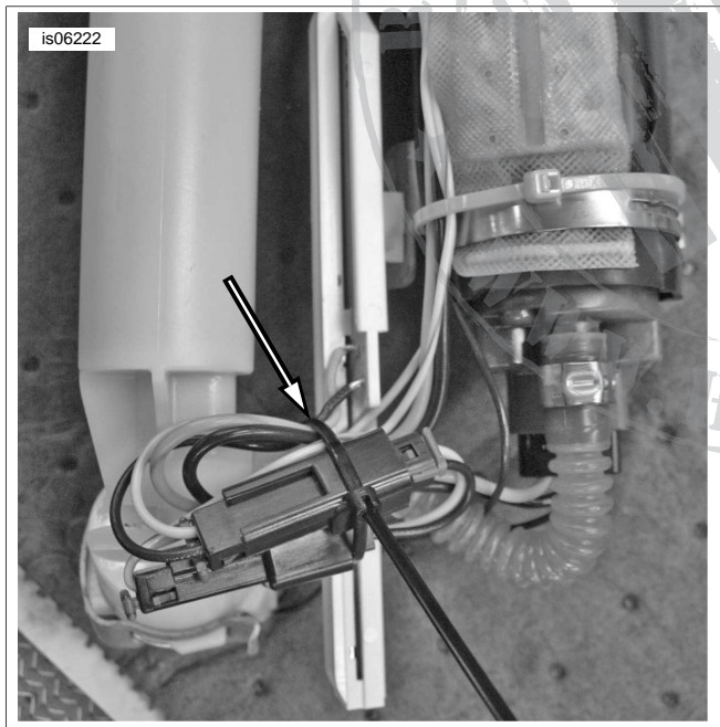
Figure 2. Secure Fuel Pump Wires and Connectors
