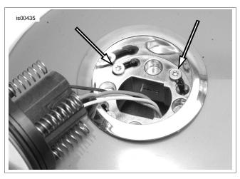
Figure 8. Gauge Housing in Unlocked Position
