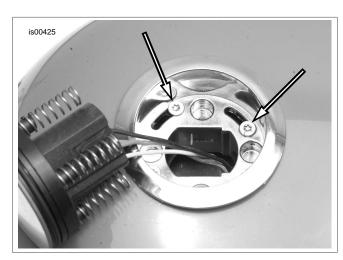
Figure 9. Gauge Housing in Locked Position
