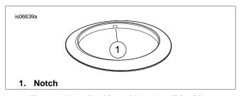
Figure 2. Note Position of Notch on Trim Ring
