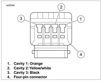
Figure 7. Four-Pin Connector (viewed from wire end)
