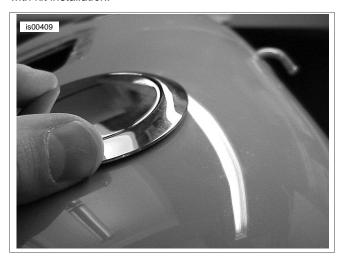
Figure 3. Determine Position for Trim Ring
