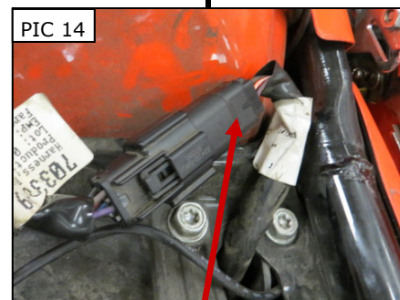
USE THE WIRES ON THIS END OF THE CONNECTOR
