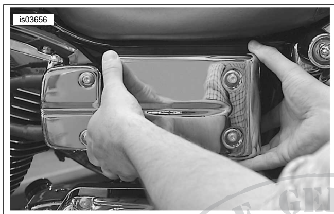
Figure 19. Electrical Caddy Cover
