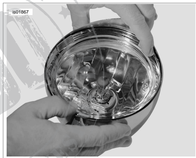
Figure 16. Chrome Trim Ring (two-sided tape shown)
