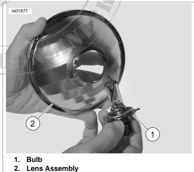
Figure 20. Lens Assembly and Bulb
