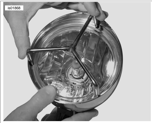
Figure 17. Service Tool and Inner Ring
