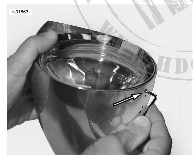
Figure 14. Allen Wrench and Outer Set Screw
