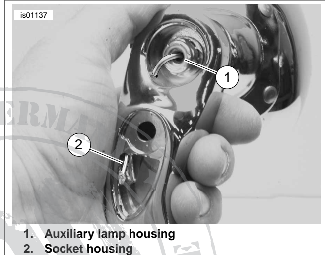
Figure 3. Auxiliary Lamp Wire Routing
