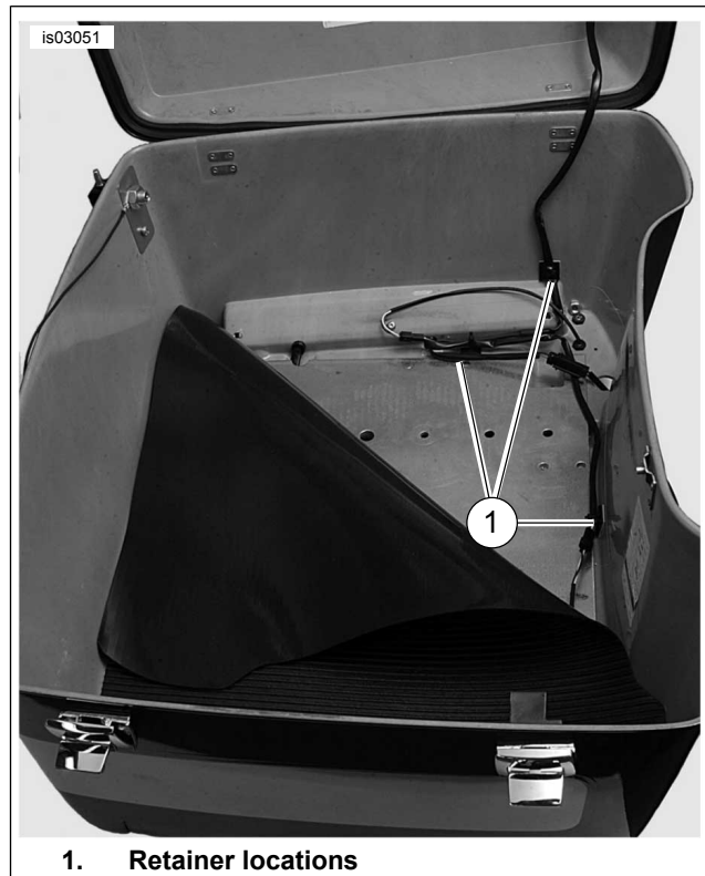
Figure 3. Suggested Wire Retainer Locations in Base
