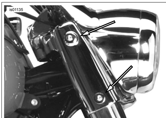
Figure 2. Typical Mounting Screw Locations (FLHRS)
