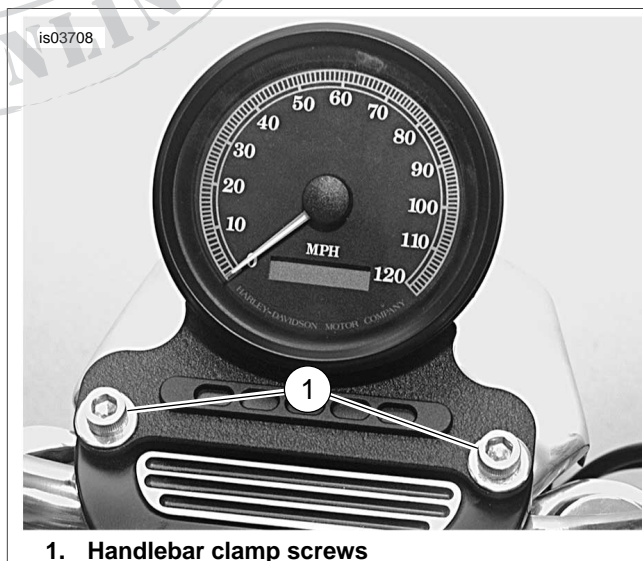
Figure 2. Remove Speedometer Bracket Assembly
