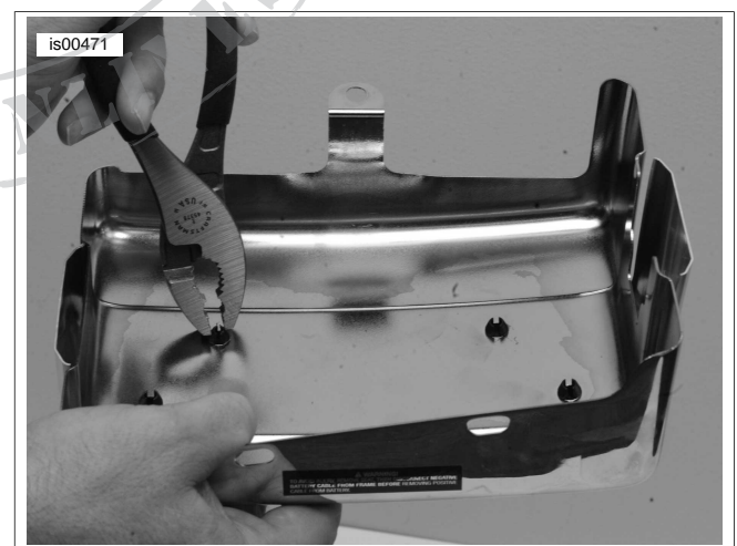
Figure 2. Push pinch tabs out of battery cover.
