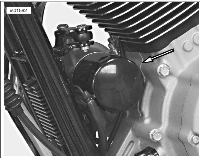
Figure 1. Spin-On Oil Filter (Sportster Evolution Engine)
