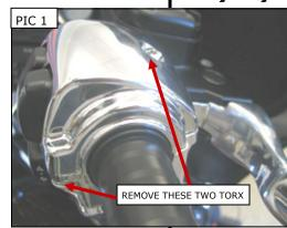
Reassemble the switch housings using the two Torx screws that were removed in STEP 2. Tighten the screws on the brake clamp if they were loosened.
