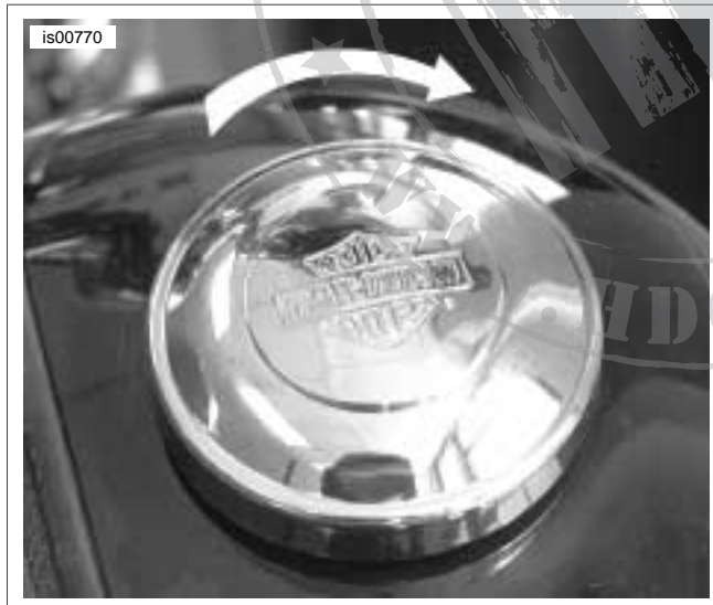
Figure 1. Right Hand Threaded Fuel Cap Installation
