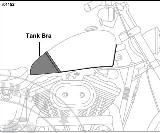
Figure 1. Tank Bra Installed (XL Standard Shown)
