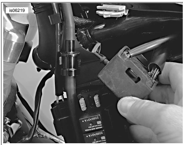
Figure 4. Converter Module Installation
