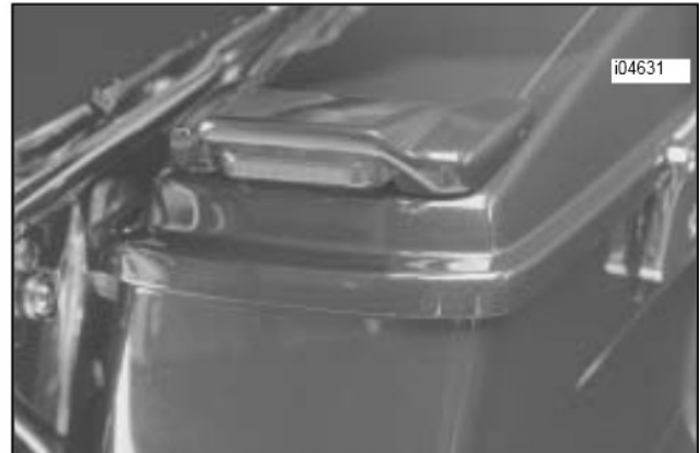
Figure 1. Installed Saddlebag lid spoiler
