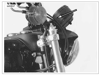
Figure 5. Cable Routing (FXD, FXDX, and FXDS-Conv Models)
