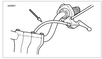
Figure 2. New Clutch Cable Routing
