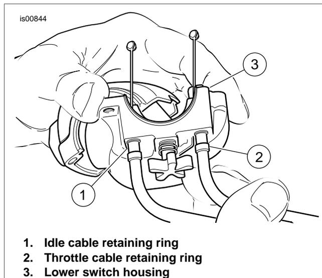
1. Idle cable retaining ring
