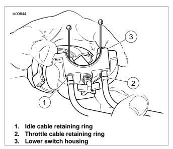
Figure 10. Install Cables to Lower Switch Housing
