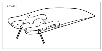
Figure 11. Windshield Mounting Brackets
