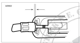
Figure 3. Clutch Cable Free Play, 1/16-1/8 in. (1.6-3.2 mm)
