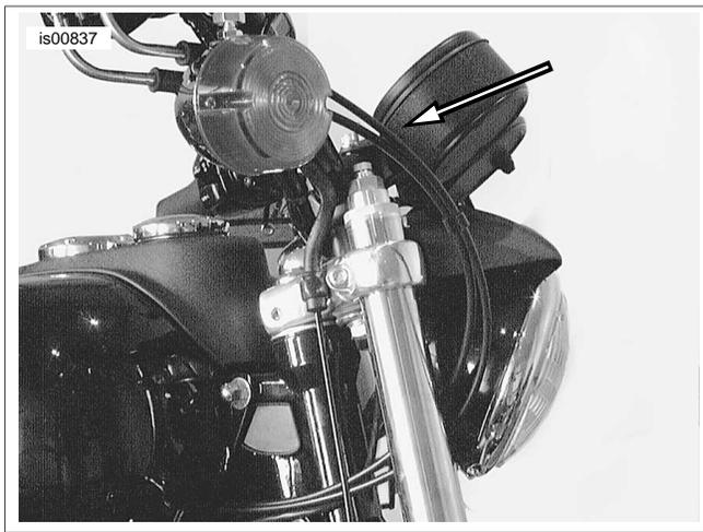
Figure 5. Cable Routing (FXD, FXDX, and FXDS-Conv Models)
