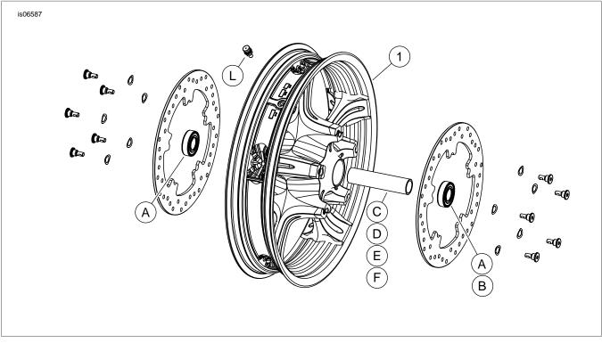
Figure 1. Service Parts: FRONT ANARCHY WHEELS (18-inch wheel shown)
