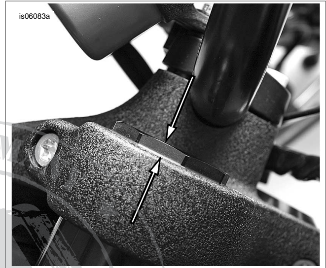
Figure 1. Fork Installation Height Measurement.
