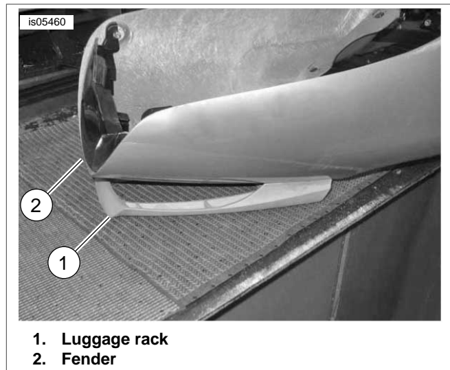
Figure 3. Align Luggage Rack and Fender
