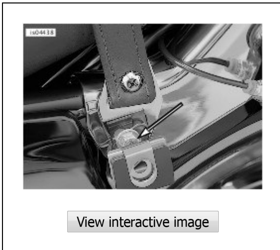
Figure 1. Passenger Grab Strap Removal (2008 Shown)
