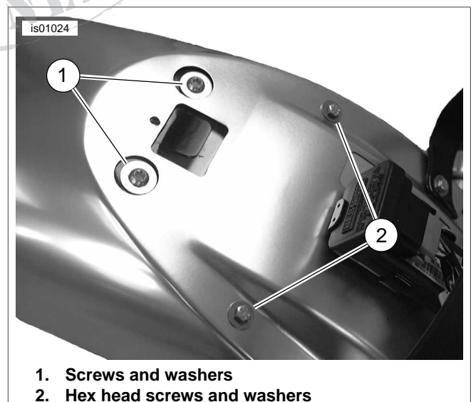
Figure 3. Remove Fender Support Screws and Washers
