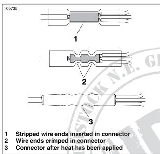
Figure 5. Install Sealed Butt Connectors
