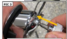
CREATE THREADS BY THREADING THE SCREW THROUGH THE BRACKET AND ALL THE WAY INTO THE INSERT ASSEMBLY; REMOVE THE SCREW AND BRACKET BEFORE INSTALLING ON THE BIKE
