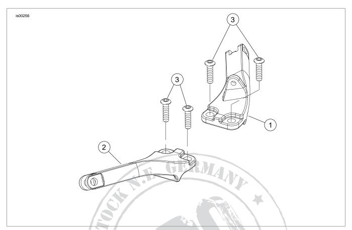
Figure 1. Passenger Support Bracket
