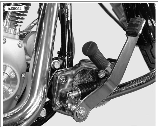
Figure 8. Extended Reach Controls - Right Side (engine guard not included in kit)
