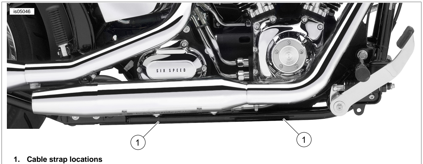
Figure 3. Cable Strap Location
