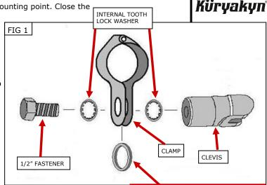
SPACER WASHER MUST BE INSTALLED **BETWEEN CLAMP HALVES! FAILURE TO** DO SO MAY RESULT IN UNSECURED CLAMPING OR DAMAGE TO THE CLAMP.
