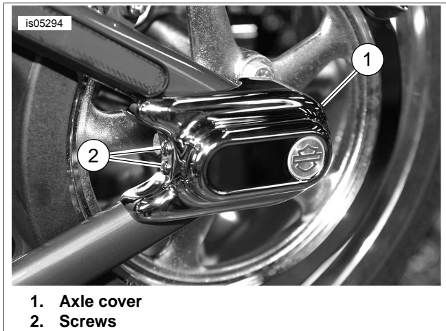
Figure 3. Axle Cover Installed
