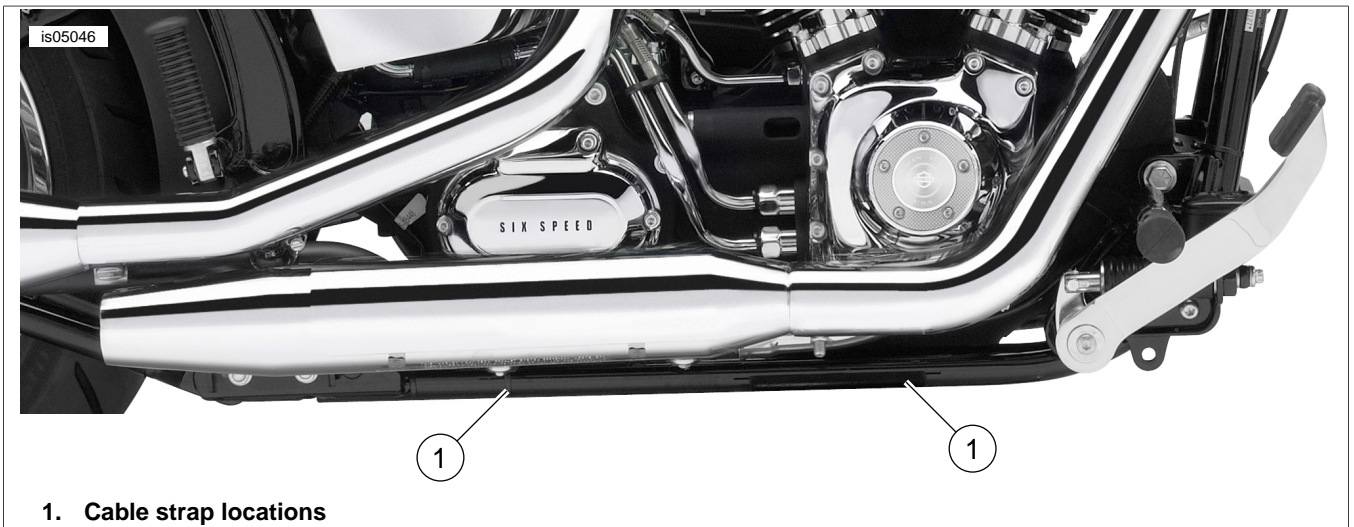
Figure 3. Cable Strap Location
