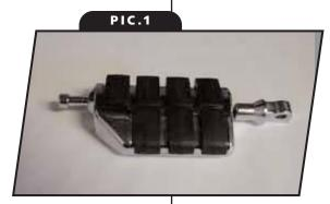
**STEP 2** Find the correct stirrup assembly for each side of the bike — the heel rest platform should face in the same direction as the footpeg.
