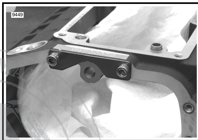
Figure 1. Install Drill Plate to Transmission Case
