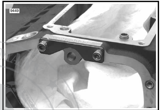
Figure 1. Install Drill Plate to Transmission Case
