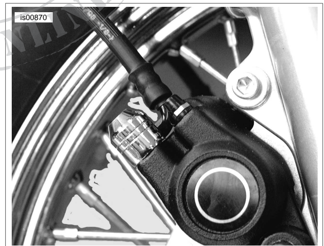
Figure 3. Installed Banjo Bolt Cover
