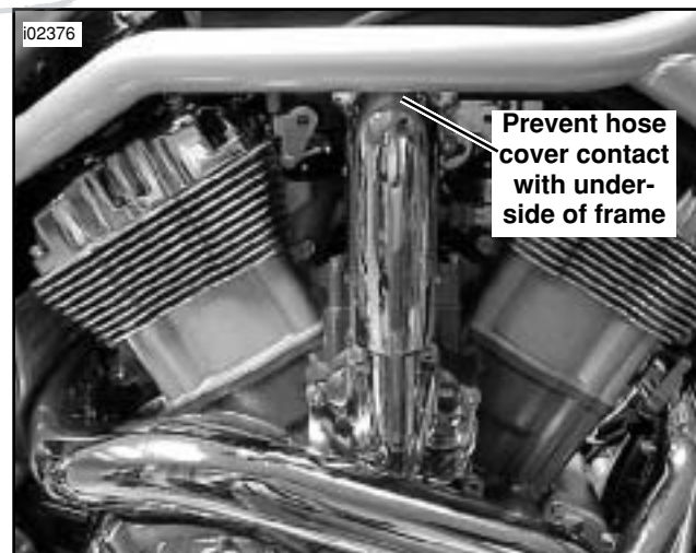
Figure 3. Hose Cover Installed
