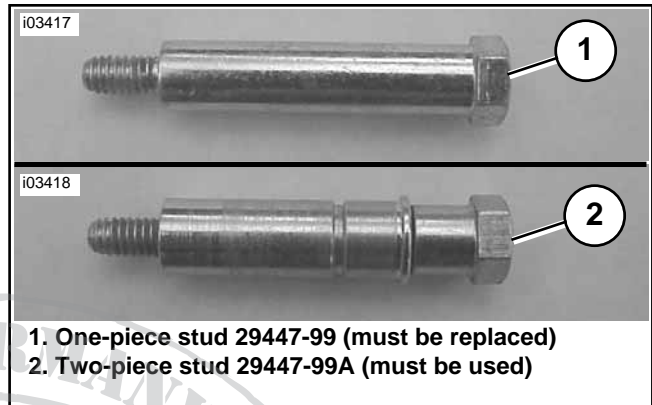
Figure 2. Two-Piece Studs MUST Be Used
