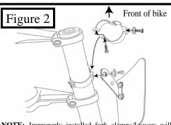
NOTE: Improperly installed fork clamps/Lowers will cause damage to your motorcycle. Make sure that the fork clamps/Lowers clear the fender, gas tank and all accessories.
