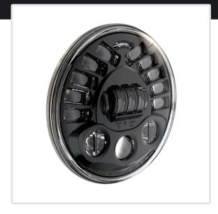
**Description** 12V SAE/ECE LED High & Low Beam Headlight with Black Inner Bezel
