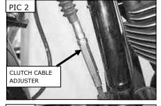
STEP 10 Refer to PIC 2. Loosen the clutch cable adjuster so the maximum amount of slack is attained. Pull the cable housing as far out of the clutch perch as possible (PIC 3) and rotate the cable and housing away from the handlebar (PIC 4). The lever may now be pulled free of the perch (PIC 5).
