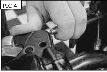
Apply a small amount of grease to the pivot pin; ensure the nylon bushing is in place in the new lever; reassemble in reverse order of disassembly.
