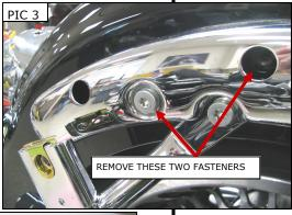
WARNING BOTH PIVOT/HINGE SCREWS MUST HAVE THREADLOCK COMPOUND RE-APPLIED AND RE-TORQUED ONCE REMOVED
