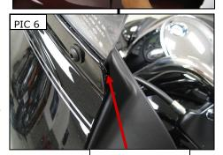
ROUTE WIRES BETWEEN THE FAIRING HALVES ON **BOTH SIDES**
