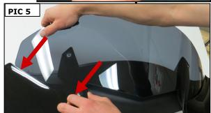
Step 7 Secure the windshield with the four screws and Spacers; ensure that the Spacers remains in place and the screw shoulders fit all the way in the hole as they are tightened.
