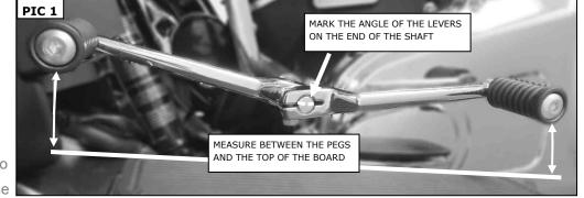
existing shift levers on the end of the shift shaft.
